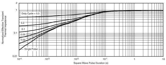
Normalized Thermal Transient Impedance, Junction-to-Foot
