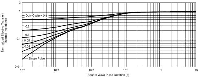
Normalized Thermal Transient Impedance, Junction-to-Foot
