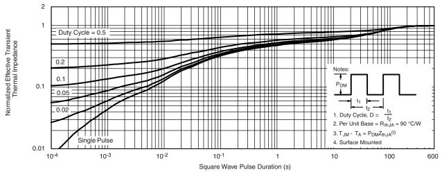
Normalized Thermal Transient Impedance, Junction-to-Ambient
