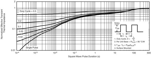
Normalized Thermal Transient Impedance, Junction-to-Ambient
