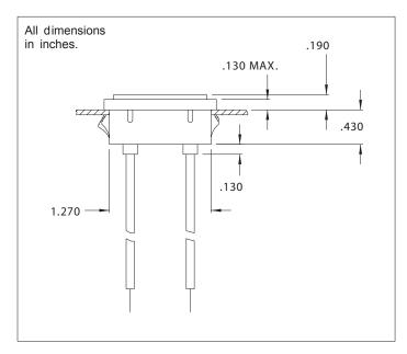
Mounting: Will snap-fit into  $\emptyset$ .032/.100 thick panels. Use speednut for other panel thicknesses.
