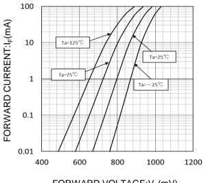
$\begin{array}{l} {\sf FORWARD\ VOLTAGE:} {\sf V_F(mV)} \\ {\sf V_F-I_F\ CHARACTERISTICS} \end{array}$
