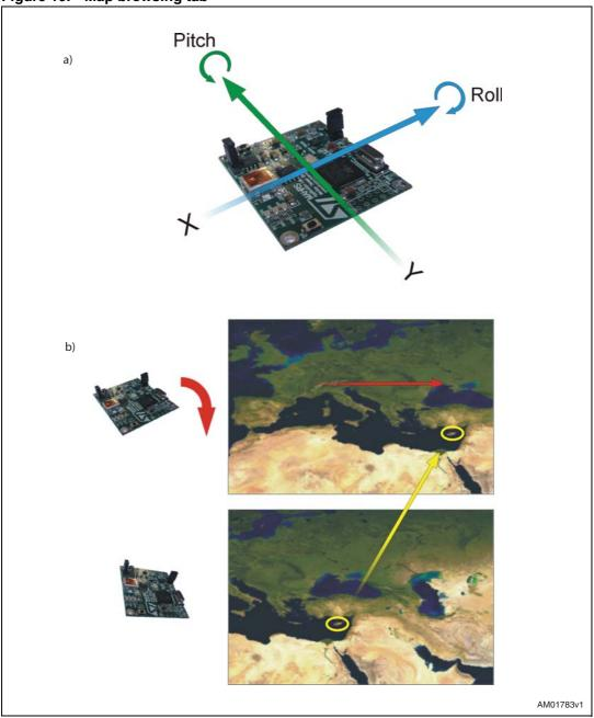
To move the map on the screen, the user must tilt the demonstration kit.
