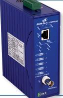
• Line port link is full-duplex up to 85Mbps over existing coaxial cable .
