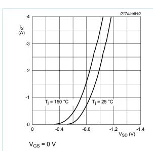
Fig. 18. MOSFET transistor: Source current as a function of source-drain voltage; typical values
