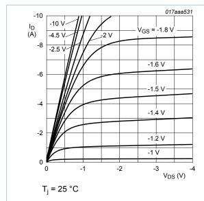
Fig. 8. MOSFET transistor: Output characteristics: drain current as a function of drain-source voltage; typical values
