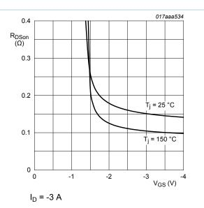
Fig. 11. MOSFET transistor: Drain-source on-state resistance as a function of gate-source voltage; typical values
