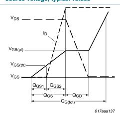
Fig. 17. MOSFET transistor: Gate charge waveform definitions
