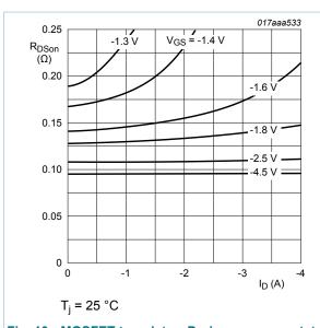
Fig. 10. MOSFET transistor: Drain-source on-state resistance as a function of drain current; typical values
