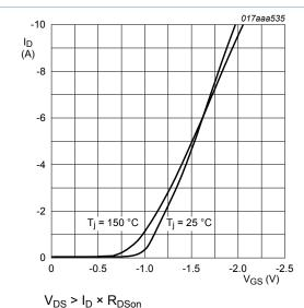
Fig. 12. MOSFET transistor: Transfer characteristics: drain current as a function of gate-source voltage; typical values
