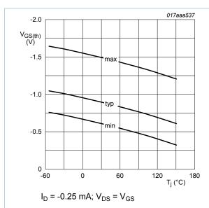
Fig. 14. MOSFET transistor: Gate-source threshold voltage as a function of junction temperature
