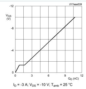
Fig. 16. MOSFET transistor: Gate-source voltage as a function of gate charge; typical values
