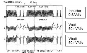
Figure 7. Load Transient Response Rlim=2.5K (Vin = 1.3V, Vout = 3.3V)
