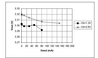
Figure 3. Line/Load Rejection Vs Output Current (Vout = 3.3V) Rlim=2.5K
