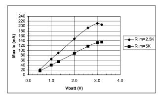
Figure 6. Maximum Load Current Vs Vbatt (Vout = 3.3V)
