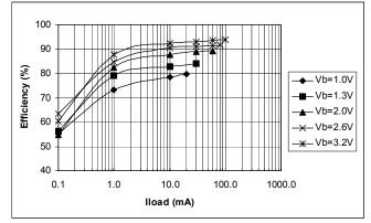
Figure 2. Efficiency Vs Output Current (Vout = 3.3V) Rlim=5K
