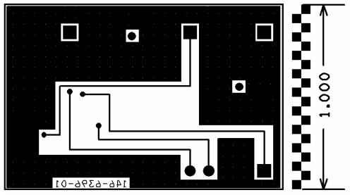
FIGURE 11: SP6644/6645UEB PC LAYOUT BOTTOM SIDE
