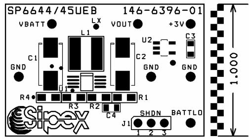
FIGURE 9: SP6644/6645UEB COMPONENT PLACEMENT
