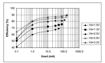
Figure 1. Efficiency Vs Output Current (Vout = 3.3V) Rlim=2.5K
