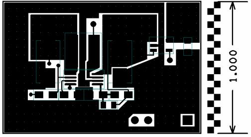
FIGURE 10: SP6644/6645UEB PC LAYOUT TOP SIDE
