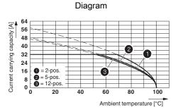
Derating curve for: IPC 5/...-ST-7,62 with IPC 5/....-G-7,62 Conductor cross section 6  $\rm mm^2$
