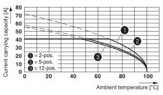
Derating curve for: IPC 5/...-ST-7,62 with IPC 5/...-G-7,62 Conductor cross section =  $10 \text{ mm}^2$
