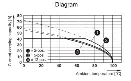
Derating curve for: IPC 5/...-ST-7,62 with PC 5/...-ST-7,62 Conductor cross section = 10 mm<sup>2</sup>
