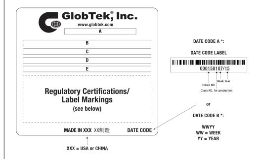
A=Medical/ITE/Household use Power Supply B=P/N: (料号) TR9CE3000T00-IMR6B C=Model (型号) GTM96300-3614.5-2.5-T3 D=Input (输入) 100-240V~, 50-60 Hz, 1A E=Output (输出)12 V === 3.0 A ,36.0W
