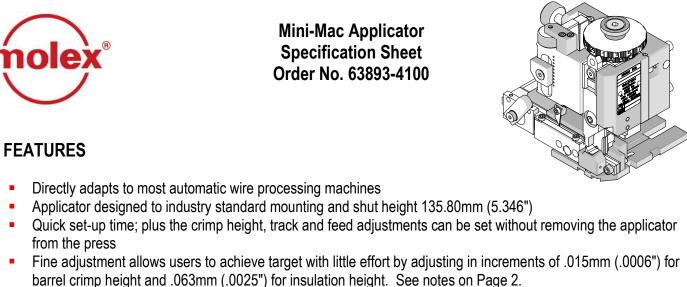
Independent adjustment rings allow users to guickly adjust the barrel or insulation crimp height without affecting each other.
