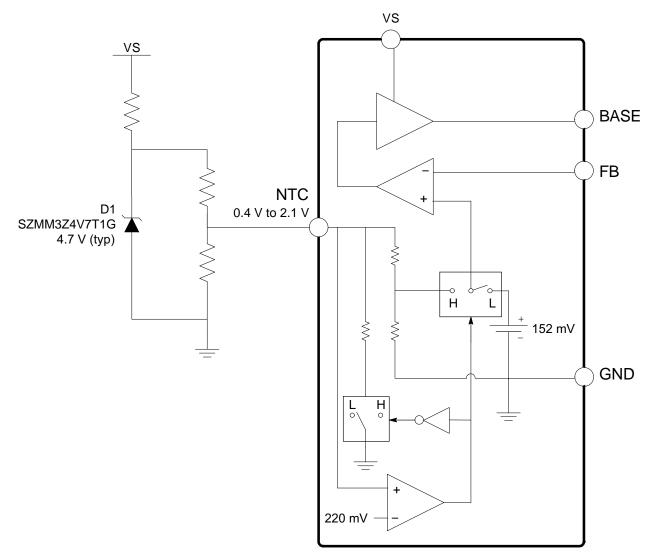
Figure 11. Negative Temperature Compensation Operation
