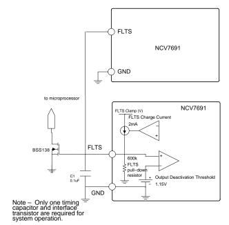
Figure 10. FLTS Wired OR to Microprocessor
