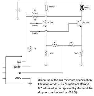
Figure 20. Open Circuit
