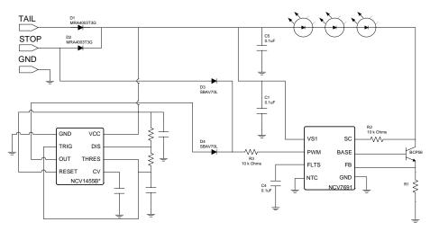
Figure 17. Stoplight / Taillight Application at higher currents
