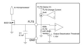
Figure 9. Open Drain Output Interface to Microprocessor
