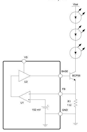
Figure 7. Output Drive Configuration
