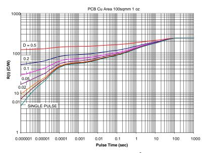
Figure 5. Thermal Duty Cycle Curves on 650 mm<sup>2</sup> Spreader Test Board
