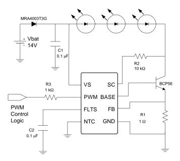
Figure 2. Microprocessor Controlled Application Diagram
