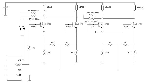
Figure 14. Saving Two Diodes for Short Circuit Protection
