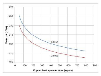
Figure 4.  $\theta_{JA}$  vs. Copper Spreader Area
