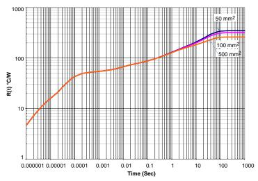
Figure 6. Single Pulse Heating Curve
