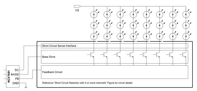
Figure 1. Application Diagram
